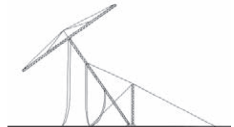
✓ Figure 3: Rotatable curtain shown in erection position
